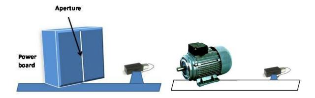
Power Boards: TEM Antenna is preferably positioned in the nearby of a Power boards apertures with the antenna aperture facing the aperture itself.
