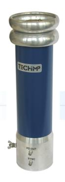
TechImp Capacitive Divider is a quadrupole suitable to **Partial** Discharge measurements. It can be chosen as detection sensor for TechImp PDSystems. By means of an internal coupling capacitor (Cc), it provides both synchronization and PD signal. The first one is filtered through a High Pass Filter, which allows test voltage rejection; the second one is filtered through a Low Pass Filter. The coupling capacitor is PD free (<2pC, 50kV, 50-60Hz).
