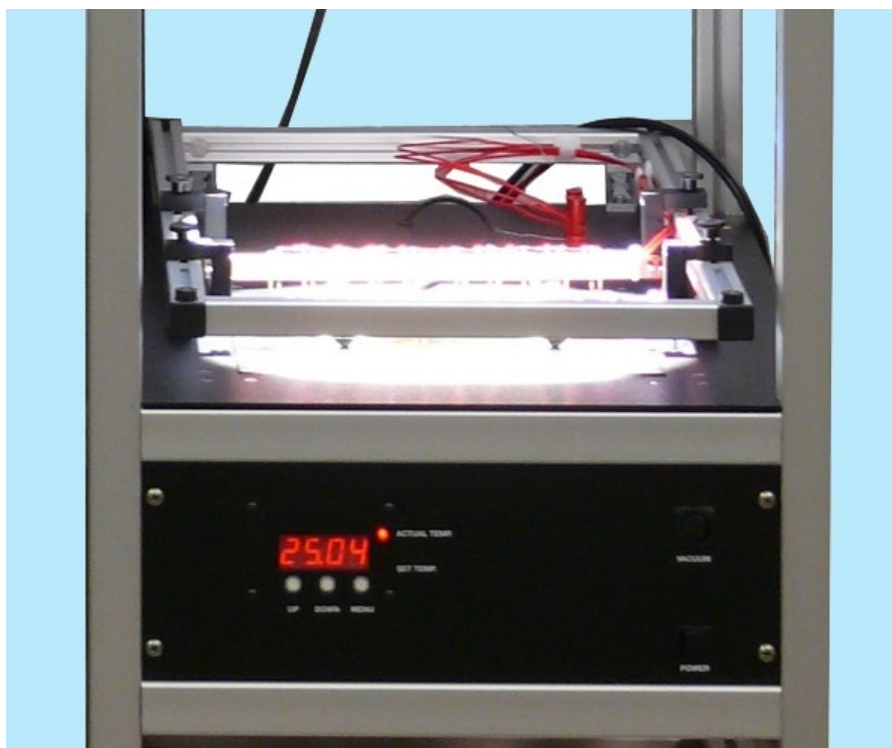
Figure 1: View of a typical cell measuring table with bottom current & voltage contacts and two (2) micro-manipulators for top cell contacts. Each Micro-Manipulator has one current & one voltage contact
