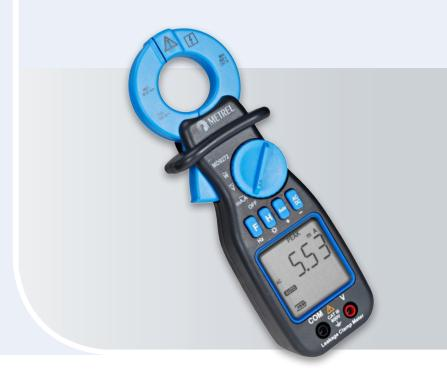
MD 9272 is a unique earth leakage clamp meter. It not just has the ability to accurately read the TRMS AC leakage current of a system, it can also detect losses in the system and suggest possible reasons for the loss. The voltage (AC/DC), frequency, power, harmonic, power factor (PF), total harmonic distortion (THD) and crest factor measurements make this instrument suitable for any electrician and engineer.
