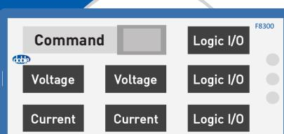
F8300 providing four phases of 150 V L-N, eight currents, and four logic I/O for testing three-phase transformer differential and transmission protection:
