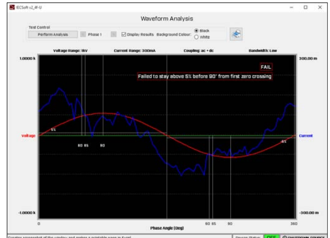
Unique “Waveform Analysis” mode, providing automated pass/fail result
