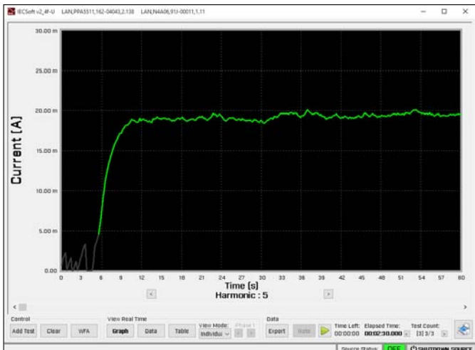
Individual Harmonics graphed, providing a deeper understanding of DUT behaviour
