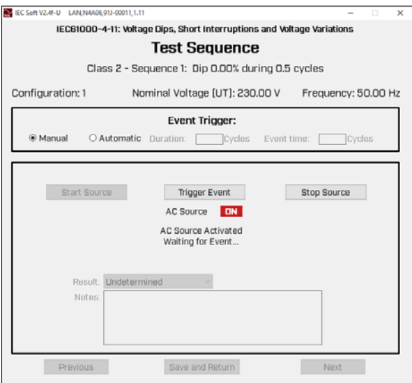
Test sequence - AC Source ON awaiting manual initiation of test sequence.
