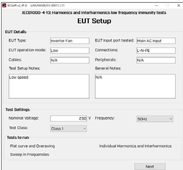
IEC61000-4-13 EUT Setup interface including class selection
