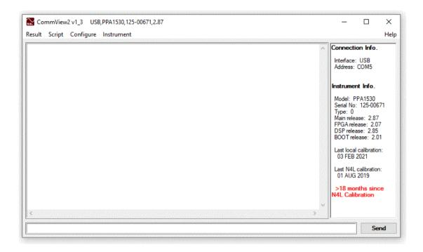
When connecting to the instrument the panel to the right hand side of the software window will display details about the instrument.
