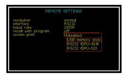
By default the save location for the screen shot will be the USB memory stick; this can be changed in the 'Remote' menu. You can change it to print to the RS232 port, that is used to print to an attached printer to print a physical copy of what is shown on the screen described in 5.10.
