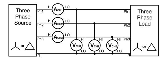
On a multi phase instrument, all the phases usually use the same input control data – internal/external, scaling factor etc. It is possible to select 'independent' so that the phases can be set up differently. This is useful if different scaling factors are required for external shunts or if one phase is using internal shunt when others are external.
