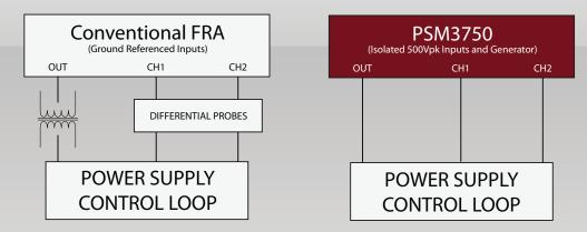
As illustrated above, the PSM3750 eliminates the requirement for an isolation transformer and differential probes. Another disadvantage when using conventional FRA instruments whilst performing analysis over a wide frequency band is that many different isolation transformers will be required for the different frequency ranges of the test. The PSM3750 eliminates this problem and generates frequencies throughout its entire frequency range from a single output.
