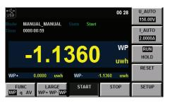
The integration function is useful for analyzing bought and sold electrical energy of a grid tied power systems. The 5335C meter provides current integral and active power integral (Wh) functionality using automatic range switching for accurate measurement results.
