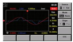
Displays waveforms of sampled voltage and current.
