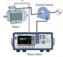
Many industrial products use PWM as a speed control method. The 5335C is able to measure input signals ranging from 0.5 Hz - 100 kHz and input voltages up to 600 V. Current can be monitored directly or by using external industry standard sensors.
