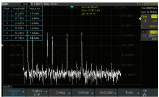
Displays signal in the frequency domain to ease measuring wave harmonics or discovering applications potential noise induced by frequency dependent components.
