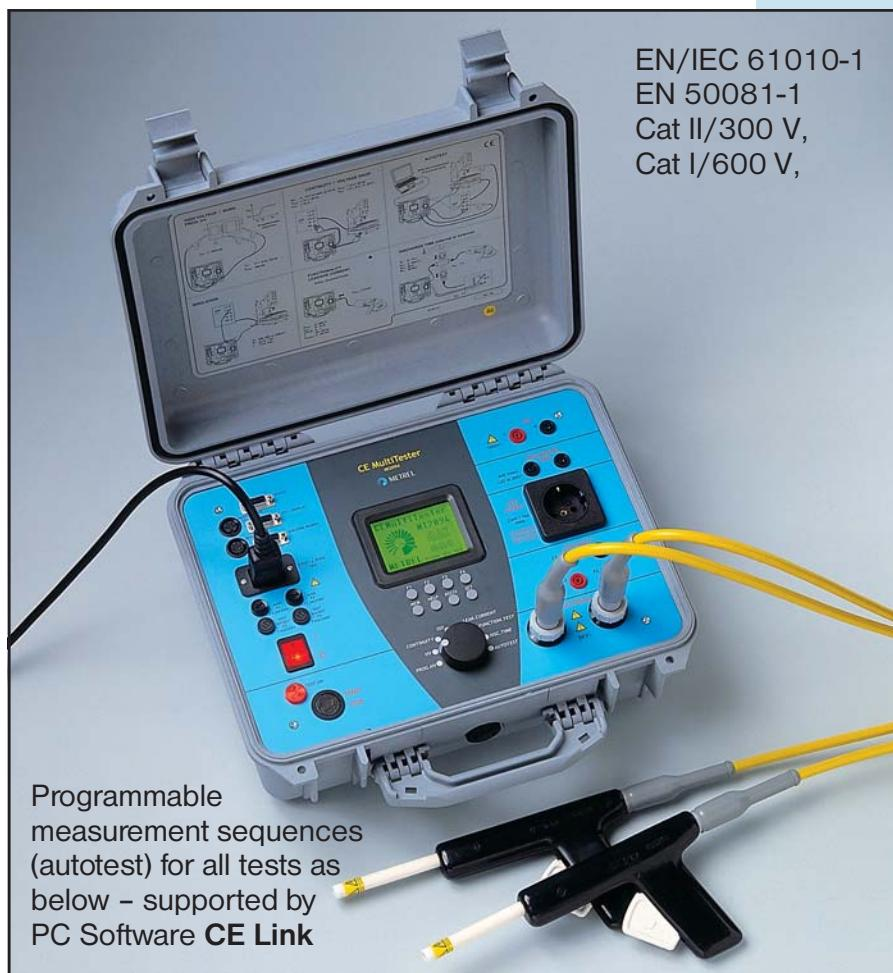
Portable, multipurpose instrument for measurements in accordance with:
