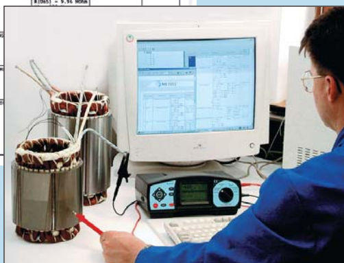
Diagnostic test of motor windings
