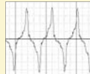
Current waveform of the switching power supply (primary side)
