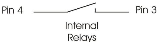
The contact is open when the system is Safe.
