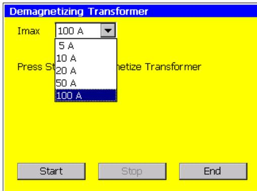
Select the demagnetizing current which is usually the same current as the test current and then press start.
