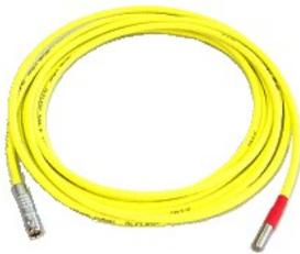
TP01 temperature probe is mounted to a flexible cable that plugs into the rear panel of the WR-instruments. This option enables the user to record the ambient temperature and/or the actual temperature of the device under test. A set of three (3) temperature probes (TP03) can be ordered to allow complete temperature measurements at three different reading points.
