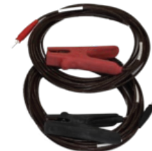
Potential cables: Channel 3 (with WR50-13R)
