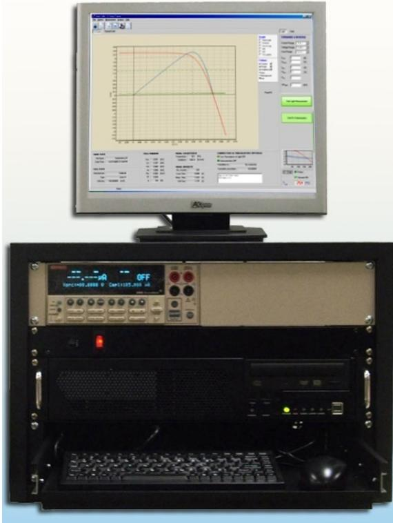
Figure 2: Typical I-V System Console
