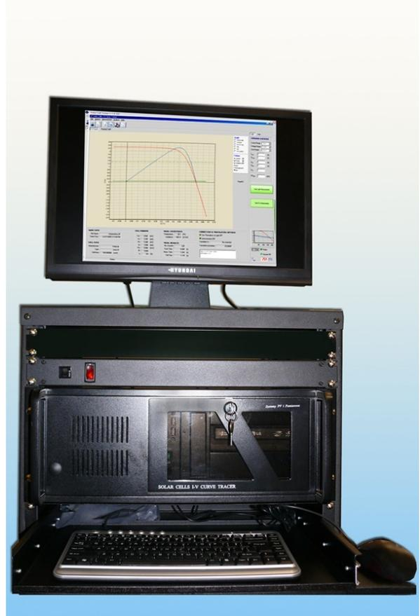
Figure 3: Typical I-V System Console
